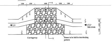
150mm Grouted Stone Pitching (Cement mortar 1:4)
