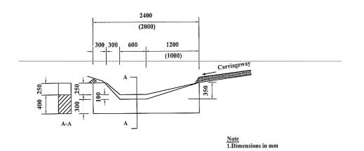
SECTION OF MASONRY SCOUR CHECK
