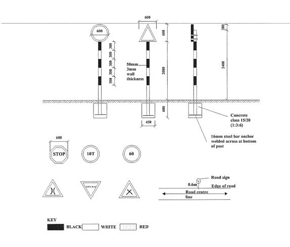
1. The type of sign required and their location shall be as shown on the Road Plan or as directed by the Engineer. 2.Sign plate to be 2mm thick mild steel plate
