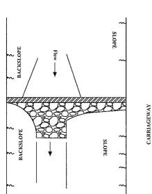
PLAN OF DRAIN WITH SCOUR CHECK
