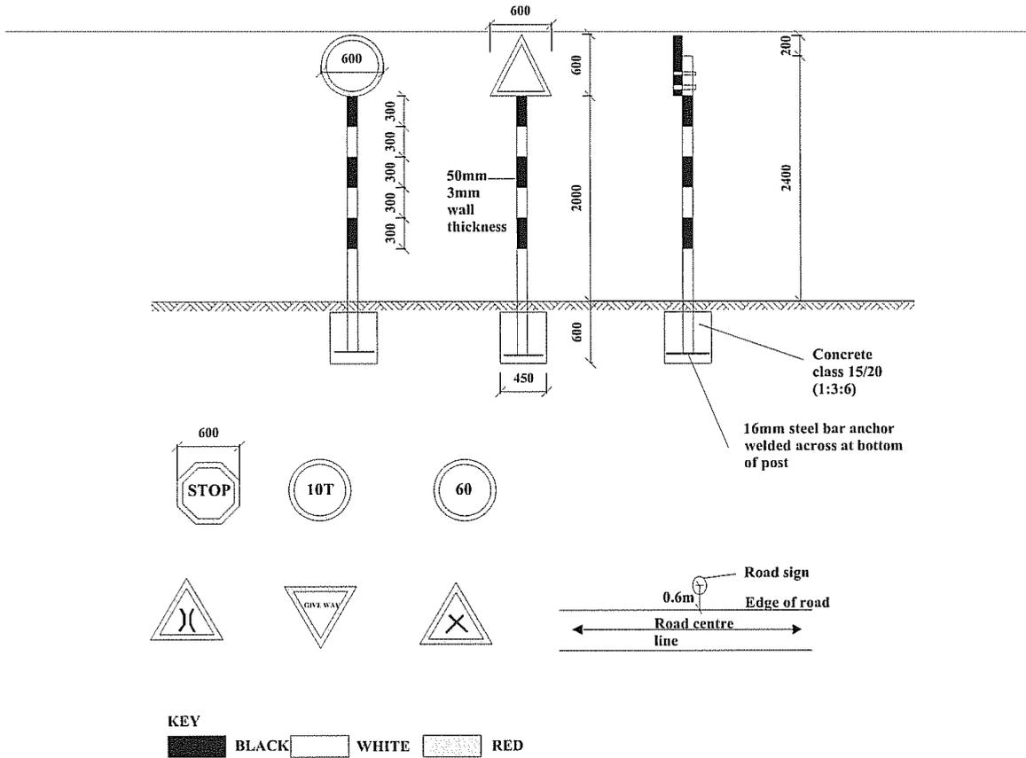
1. The type of sign required and their location shall be as shown on the Road Plan or as directed by the Engineer.
